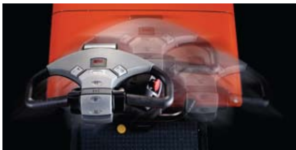
The E-man mini-tiller arm can be offset to either side (option) for easier reversing and walk-with operation
