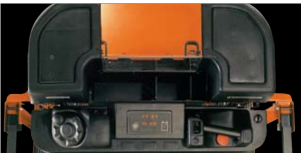
LED indicators and the digital display allow rapid fault diagnosis
